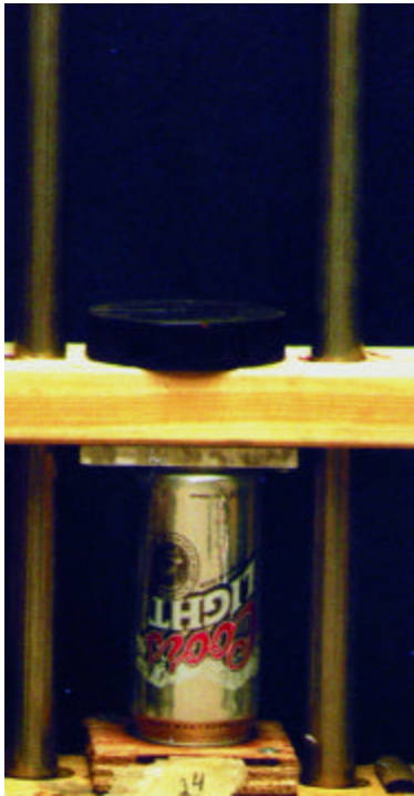
Fig. 1. Apparatus to crush aluminum cans in order to measure acceleration as a function of distance from the impact site. Steel posts mounted on lab stands serve as guide rails on which a wood board falls under gravity. Kilogram masses are affixed to top of wood board; hard metal surface applied to bottom of board creates a rigid impactor.
