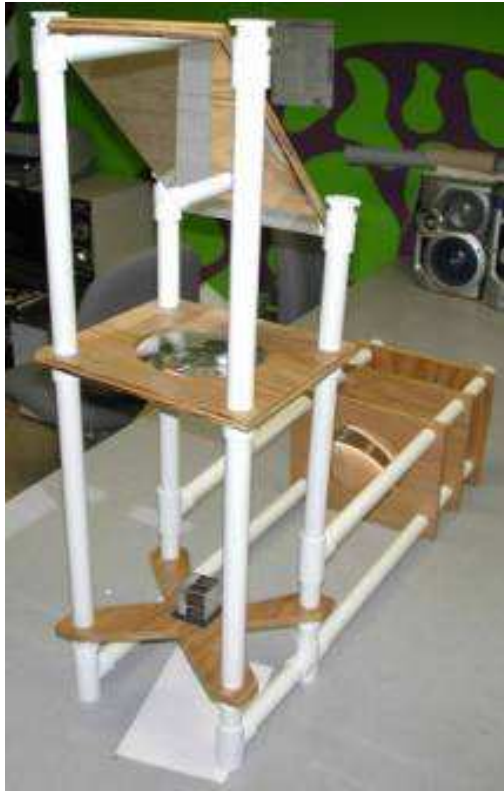
Figure 4. Left: The apparatus to demonstrate a Shack-Hartmann Wavefront sensor. The upper mirror is used merely to reflect a horizontal lightpath into the system. Right: The lens array which forms the heart of the sensor. Each samples a portion of the wavefront, projecting a displaced image on the viewing screen.
