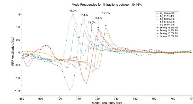
**Fig. 2:** Lowest Mode Frequencies and fill fractions. Both lab and flight (0-g) data are shown.
