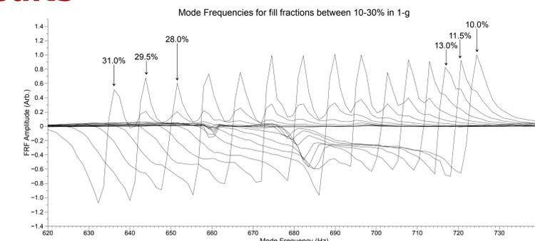
**Fig. 1:** Selected FRF data for fill levels between 10 and 31% of the tank volume in 1-g.
